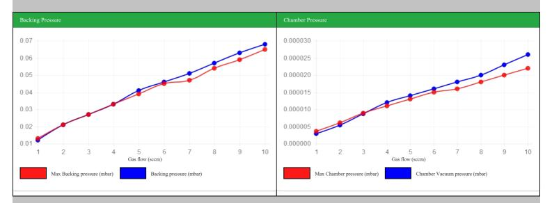
Pass critera: Linear relationship between vacuum pressure and gas flow. (Blue line should be below red line)
