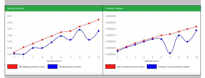
Pass critera: Linear relationship between vacuum pressure and gas flow. (Blue line should be below red line)
