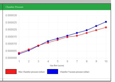
Pass critera: Linear relationship between vacuum pressure and gas flow. (Blue line should be below red line)
